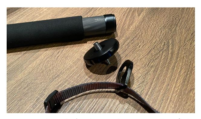
Step 1: unscrew the top plate from the monopod to gain access to the ring/eyelet where the wrist strap was attached. How the top plate detaches varies by monopod make and model. Thread safety strap tag end with the plastic buckle already on the strap through the topside of the eyelet in the monopod ring.
