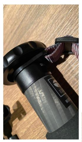
Step 3: put the ring/eyelet back on top of the monopod and screw the top plate back on top to secure the ring and top plate to the monopod.
